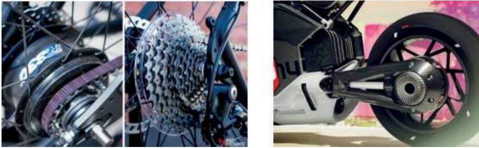
Figure 8: Belt, chains and bevel gear for power transportation for bicycle and motorcycle
